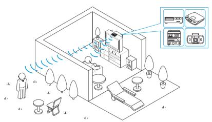
When the stethoset receiver leaves the range of the transmitter, it produces warning signals and then automatically switches off after 3 minutes.
